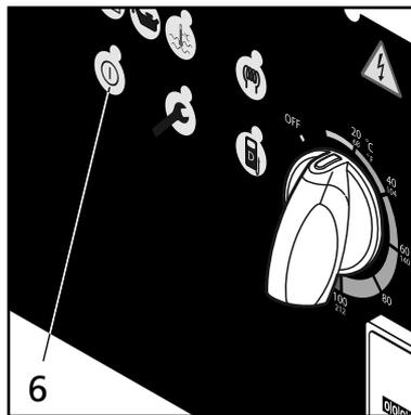
1. Turn the switch to the required temperature. Now 6 lights up and the machine is ready for use. If you want to operate with a temperature above 100°C, thurn the rotary knob (black) on the pump clockwise to limit stop.
